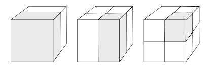
3-D domain partitioned along one (left), two (center), or all three (right) of its dimensions
