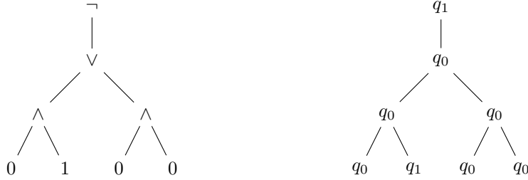
Figure 2: (a) Input tree \neg((0 \wedge 1) \vee (0 \wedge 0)) (left); (b) Run of DTA M_p on input \neg((0 \wedge 1) \vee (0 \wedge 0)) (right).
