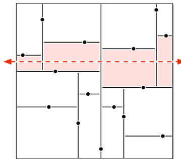
A kd-tree for 15 points. The dashed line crosses the four shaded cells.
