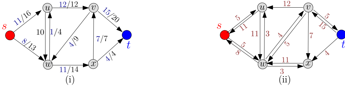
Figure 13.2: (i) A flow network, and (ii) the resulting residual network. Note, that f(u, w) = -f(w, u) = -1 and as such c_f(u, w) = 10 - (-1) = 11 .
