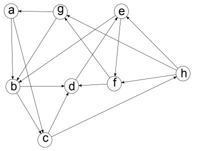
Draw the **DFS** tree rooted at d for the above graph. Use alphabetic ordering to break ties. Label the vertices of the tree with their pre(v) : post(v) time. Add in the remaining edges of the graph and label them as forward (F), backward (B), and cross (C) edges. Sort the vertices by their post visit order.
