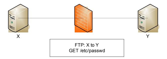
GET command causes firewall to dynamically open data channel initiate from Y to X
