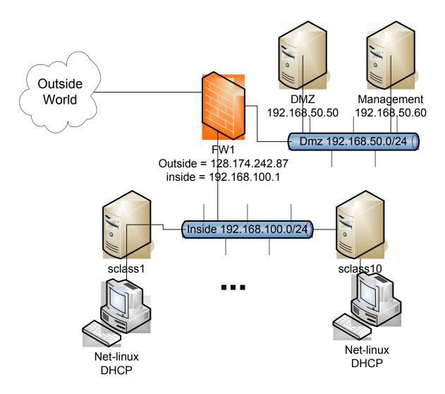
The lab has 10 dell systems. Each dell computer has Fedora Core 12 (FC12) and VirtualBox installed. The host machine is named sclassX (where X is a value between 1 and 10). The machines use DHCP to retrieve their IP addresses and DNS information from FW 1, an IOS firewall. The firewall enables connections initiated from the lab to
