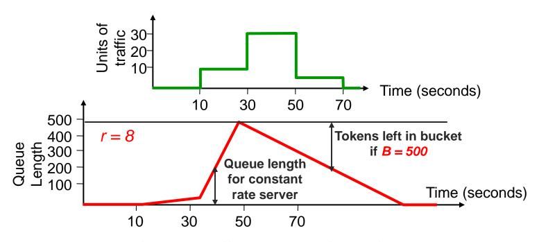
The number of empty buffer positions for buffer size B and a constant rate server is equivalent to the number of tokens in an (r,B) token bucket filter
