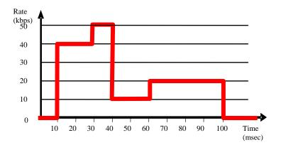
What is the minimum size of B required so that the filter lets the stream pass with no loss or delay?
