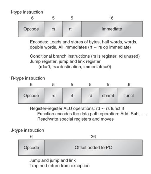
**Figure A.22 Instruction layout for MIPS.** All instructions are encoded in one of three types, with common fields in the same location in each format.
