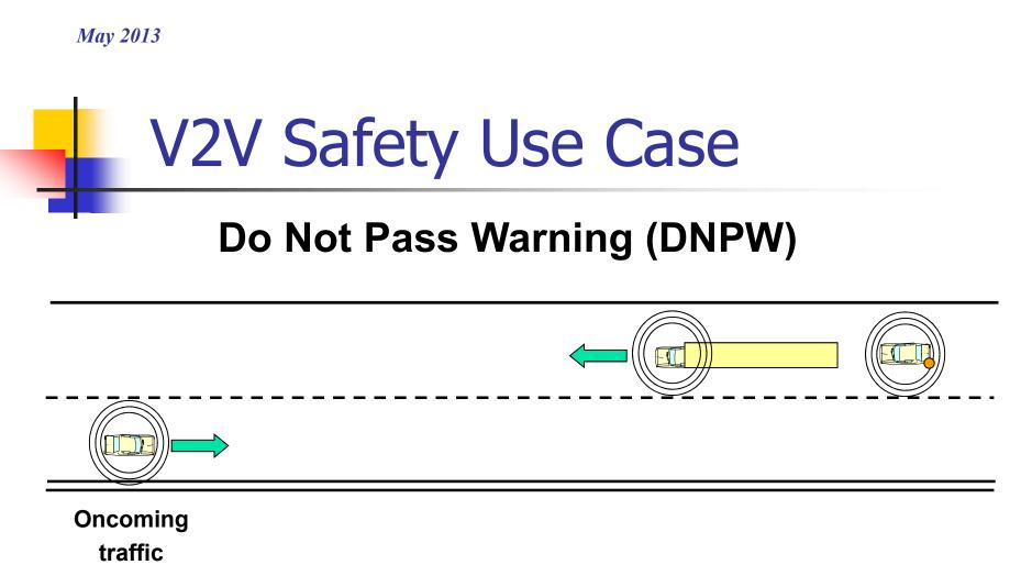
When showing intent to move to oncoming lane, driver receives warning if not safe to pass.
