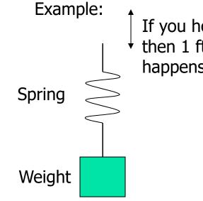
If you hold the top of the spring and move 1 ft up then 1 ft down at an increasing frequency, what happens to the range of motion of the weight?
