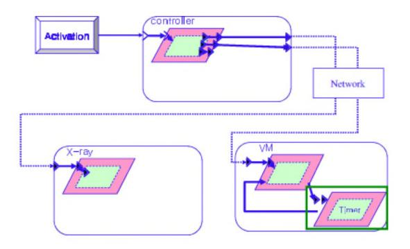
Architecture #2: Master controller on a Windows server tells ventilator when to pause. Ventilator has a hardware timer and restarts automatically once timer expires.
