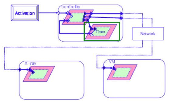
Architecture #1: Master controller on a Windows server orchestrates ventilator and X-ray machine actions over a network. Controllers tells machines to stop and re-start, and ensures that ventilator is not off too long. Comments?
