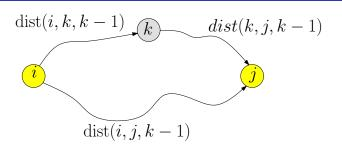
$$\label{eq:dist} \begin{aligned} \text{dist}(\textbf{i},\textbf{j},\textbf{k}) &= \text{min} \begin{cases} \text{dist}(\textbf{i},\textbf{j},\textbf{k}-1) \\ \text{dist}(\textbf{i},\textbf{k},\textbf{k}-1) + \text{dist}(\textbf{k},\textbf{j},\textbf{k}-1) \end{cases} \end{aligned}$$
