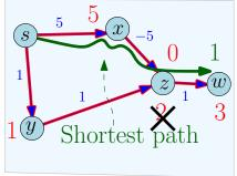
With negative length edges, Dijkstra's algorithm can fail
