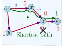
False assumption: Dijkstra's algorithm is based on the assumption that if  $\mathbf{s} = \mathbf{v}_0 \to \mathbf{v}_1 \to \mathbf{v}_2 \dots \to \mathbf{v}_k$  is a shortest path from  $\mathbf{s}$  to  $\mathbf{v}_k$  then  $\mathbf{dist}(\mathbf{s}, \mathbf{v}_i) \leq \mathbf{dist}(\mathbf{s}, \mathbf{v}_{i+1})$  for  $\mathbf{0} \leq \mathbf{i} < \mathbf{k}$ . Holds true only for non-negative edge lengths.
