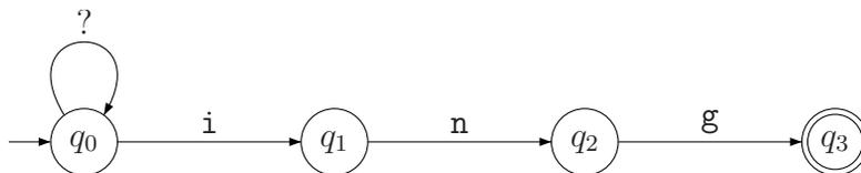
Notice key pieces of this machine: four states,  $q_0$  is the start state (arrow coming in),  $q_3$  is the final state (double circle), transition arcs.
