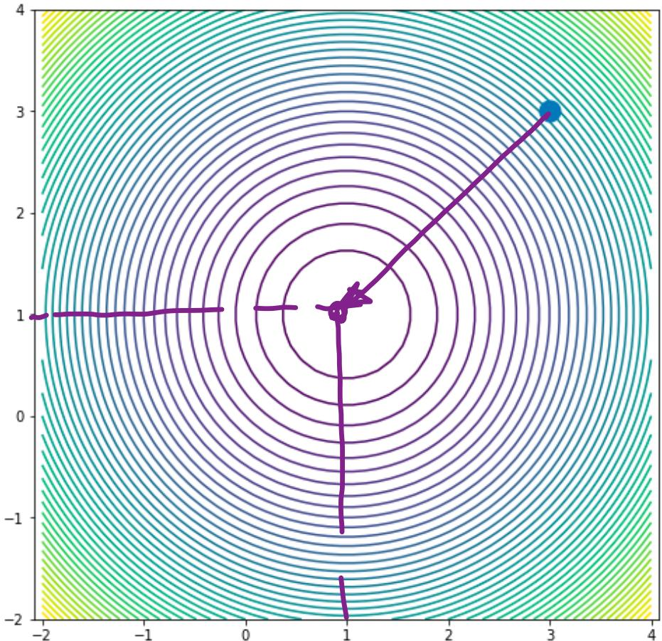
Find  $\underline{x}_1 = \underline{x}_0 - \alpha \nabla f(\underline{x}_0)$  s.t  $f(\underline{x}_1)$  is minimized
