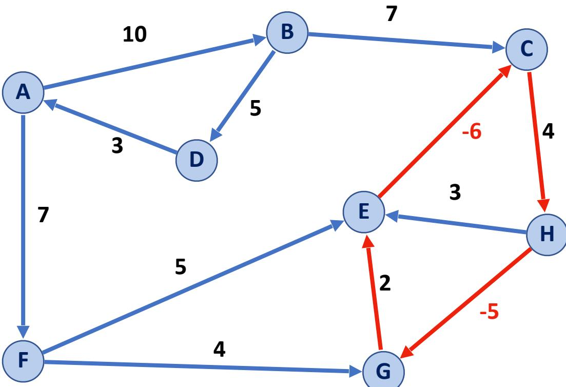
Shortest Path ( $A \rightarrow E$ ):  $A \rightarrow F \rightarrow E$   $\xrightarrow{\text{Length: 12}}$   $(C \rightarrow H \rightarrow G \rightarrow E)^*$   $\xrightarrow{\text{Length: -5 (repeatable)}}$
