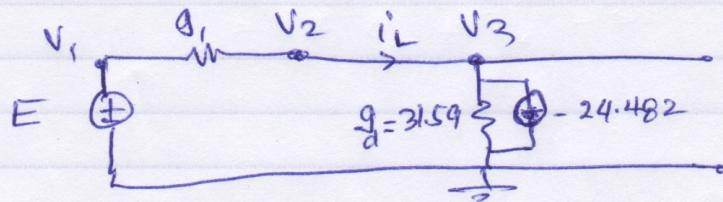
At DC, inductor is short-circuited, capacitor open.
