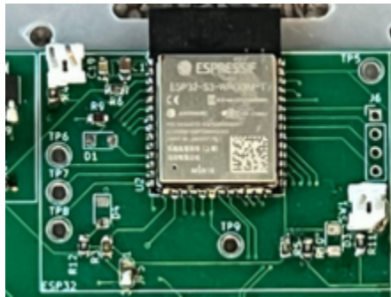
Figure 3.3 Modified PCB. Notice the white pin headers. In practice, these headers are grounded to mimic a button press.
