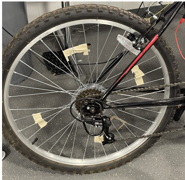
Figure 4: Placement of the magnets and Hall effect sensor on the bicycle wheel.
