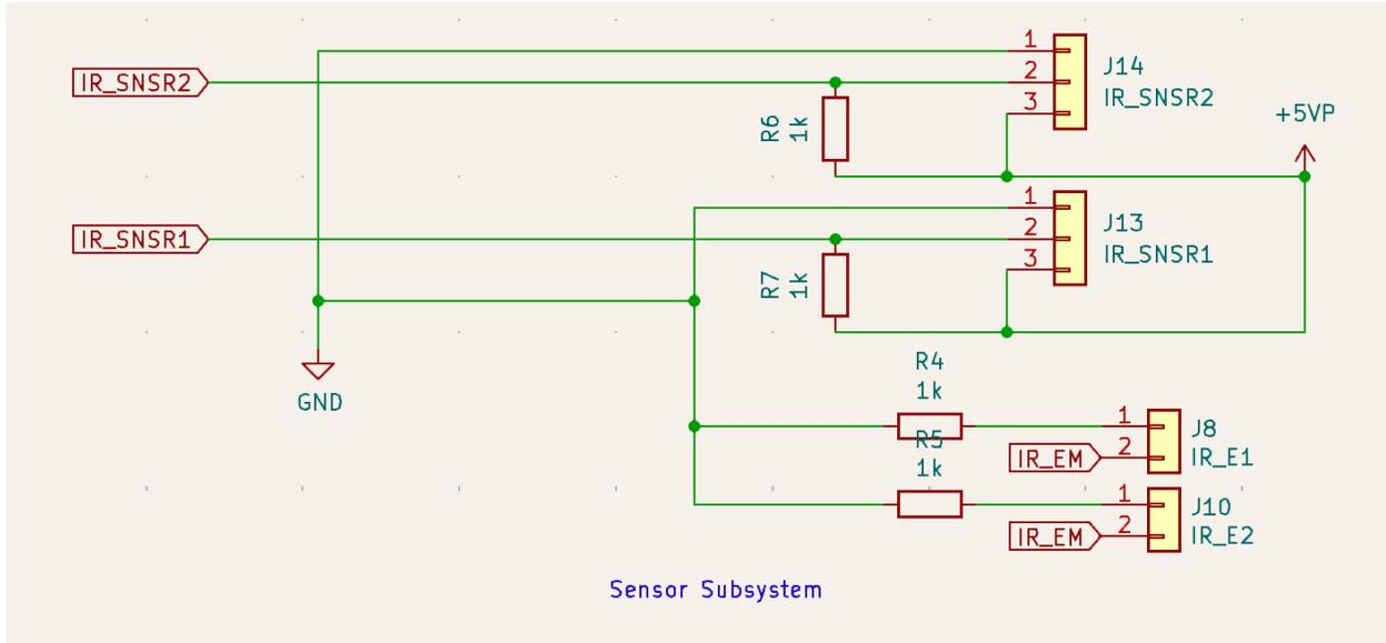
Figure 5 Sensor Subsystem
