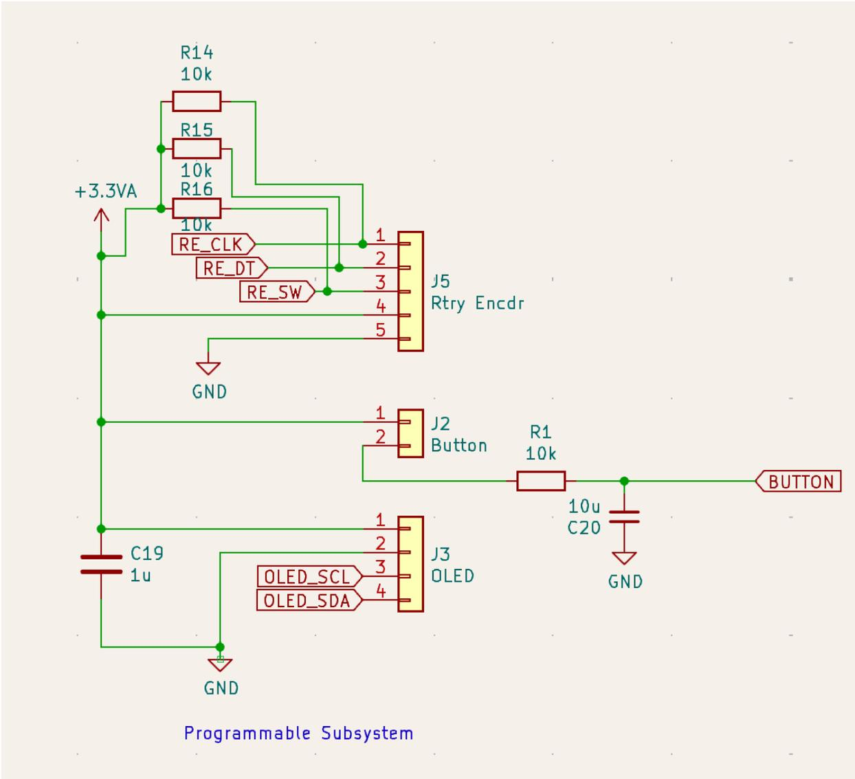
Figure 4 Programmable Subsystem
