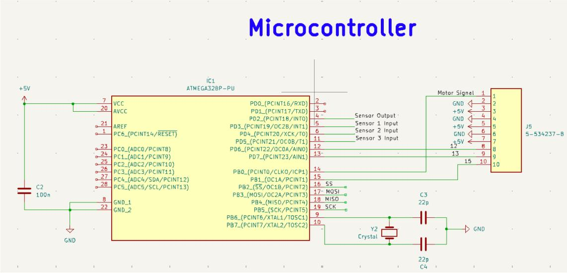
Figure 3: Microcontroller Schematic
