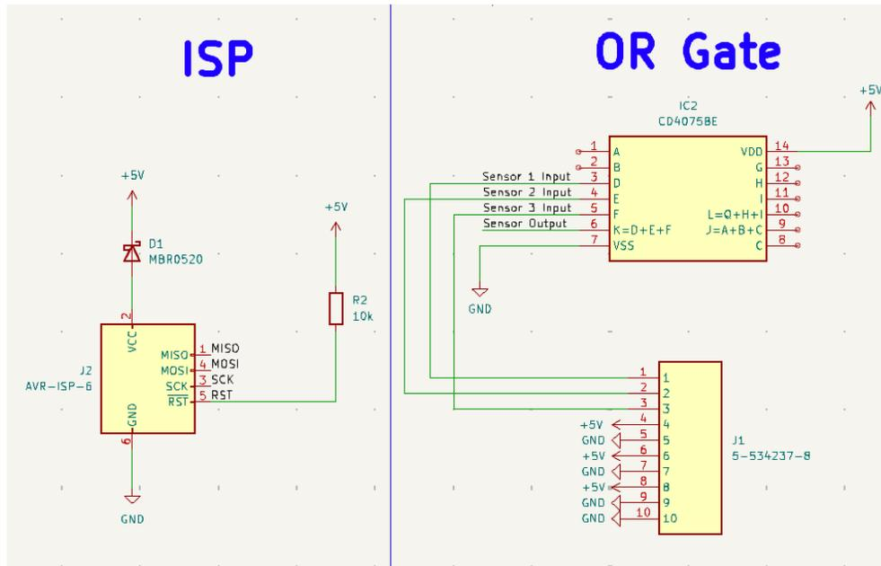
Figure 4: ISP and Triple-Or Gate Schematic
