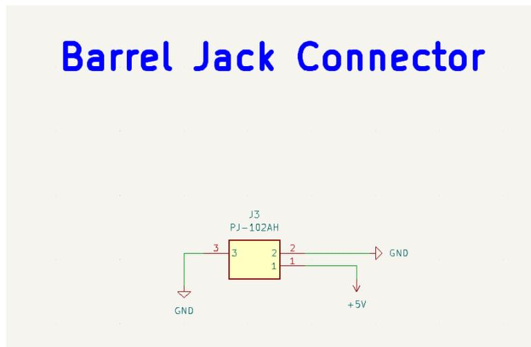
Figure 2: Barrel Jack Connector Schematic
