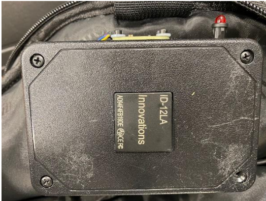
Figure 1: Final Design of Sensor and LED Case
