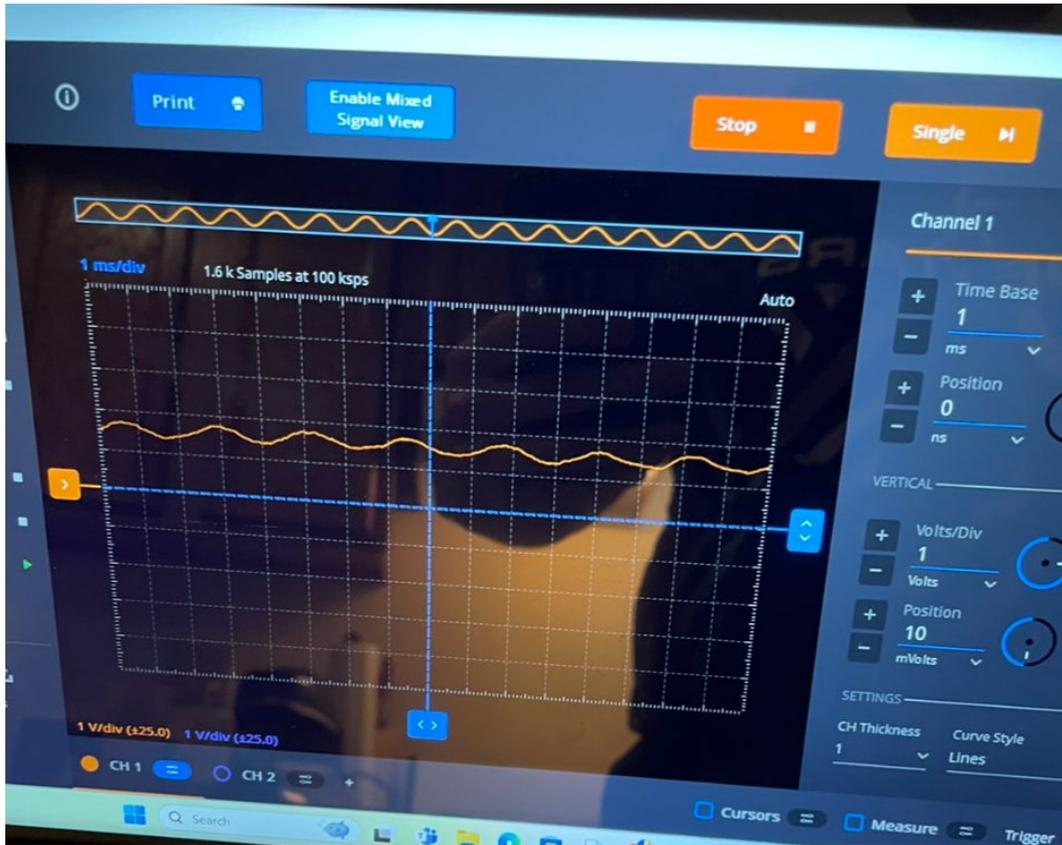
Image from oscilloscope measuring microphone receiving pure sine wave
