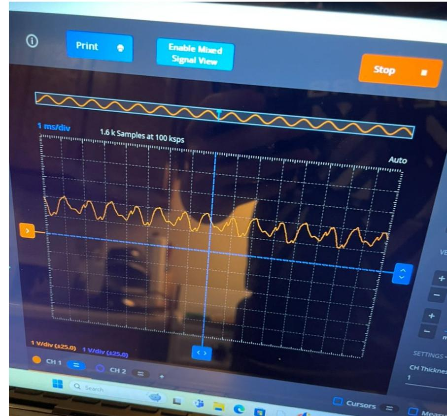
Image from oscilloscope measuring microphone receiving pure sawtooth wave
