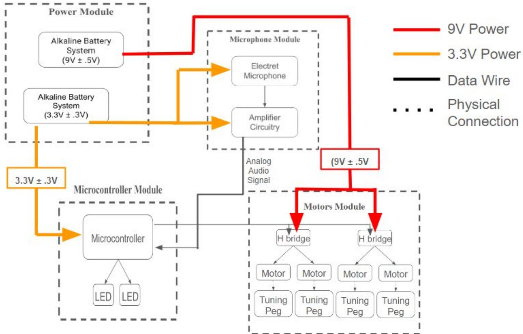
Provide consistent and accurate voltage to the other components, primarily a  $9V \pm 0.5V$  line to turn the motors and a  $3.3V \pm 0.3V$  line for most other items.
