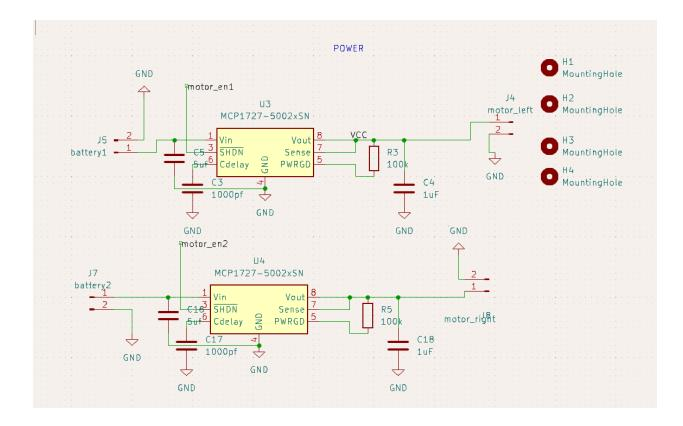
Fig 1: Power system and linear regulators
