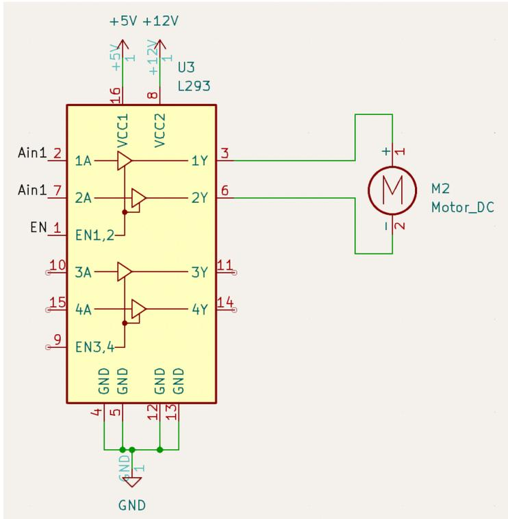
*Motor Setup for Actuator*
