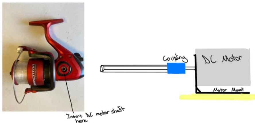
The actuator will be mounted at the tail end of the rod.
