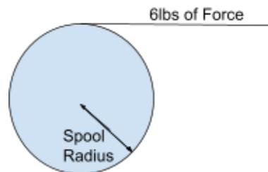
Determining the spool radius is challenging, because as the line is reeled-out the radius will decrease and as the line is reeled-in the radius will increase. We believe on average our spool's radius measures between:
