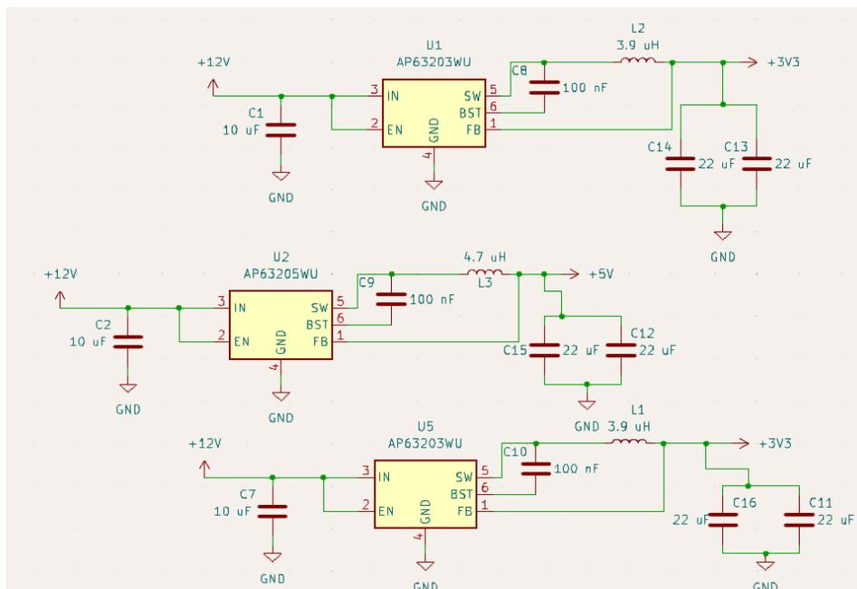
Configuration for Power Supply Subsystem
