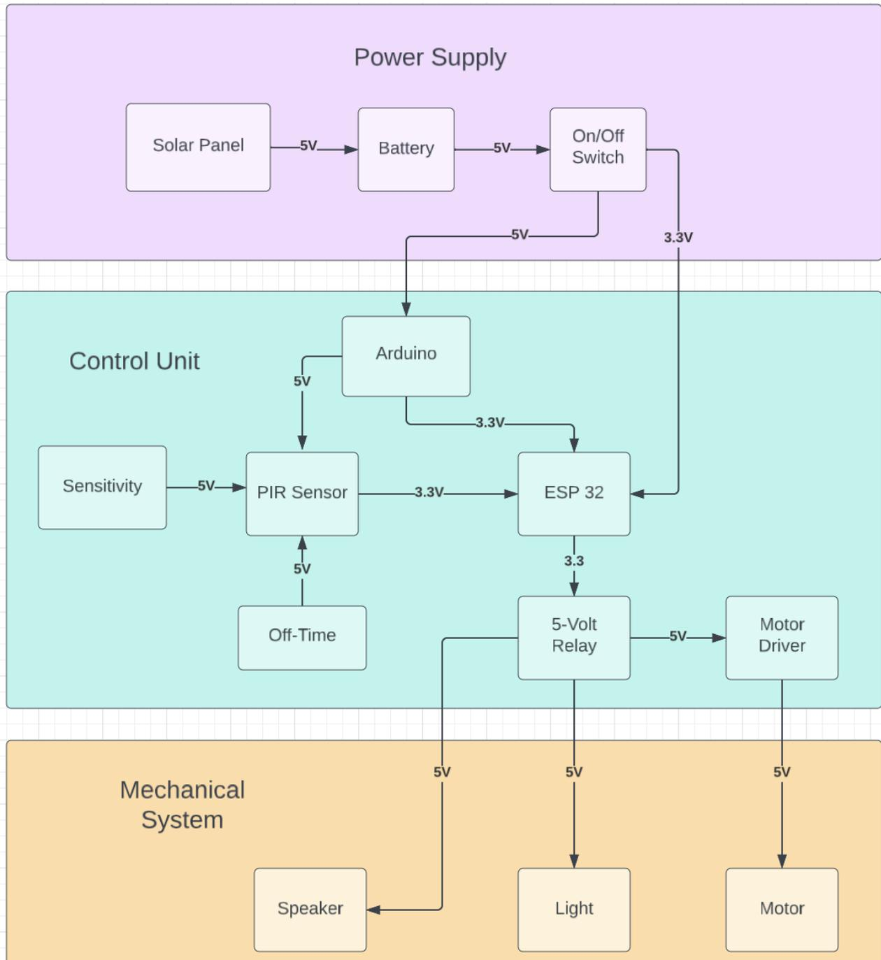
Figure 2: Block Diagram
