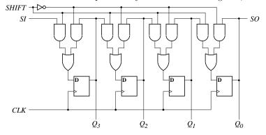
Through the use of more complex input logic, we can construct a shift register with additional functionality. The bit slice shown to the right allows us to build a bidirectional shift register with parallel load capability and the ability to retain its value
