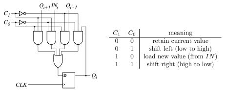
indefinitely. The two control inputs,  $C_1$  and  $C_0$ , make use of a representation that we have chosen for the four operations supported by our shift register, as shown in the table to the far right.
