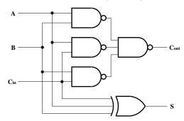
The gate diagrams above implement a single bit slice for an adder. The version on the left uses AND and OR gates (and an XOR for the sum), while the version on the right uses NAND gates, leaving the XOR as an XOR.
