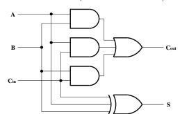
an adder bit slice using NAND gates
