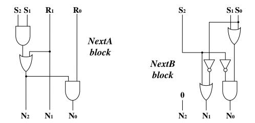
The NextA and NextB blocks are shown above. For both blocks, the S input is the current FSM state, the R input is the current fruit, and the N output is the next FSM state.
