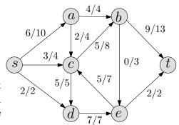
(B) Show an s-t path in the residual graph and state its bottleneck capacity. You only need to draw the path from the graph you showed in (A).
