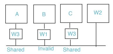
C reads W. A sees the request by snooping on the bus, asserts a signal that inhibits memory from responding, provides the values. Also changes label to Shared.
